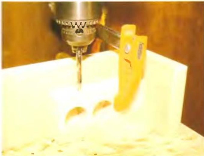
Lamination #3 in position to drill shackle retainer pin hole.
