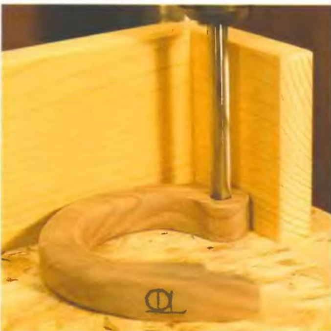
Drilling retainer pinhole in the shackle.
