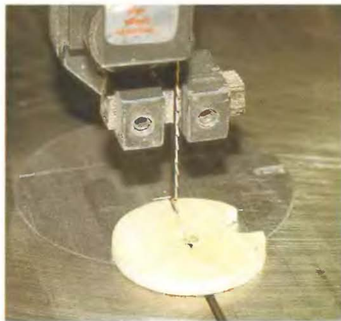
Cutting drive pin notches.
