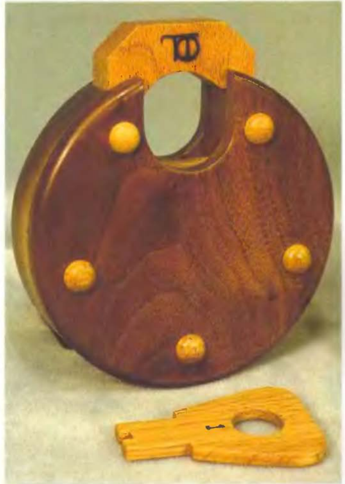
Finished push key lever lock.
