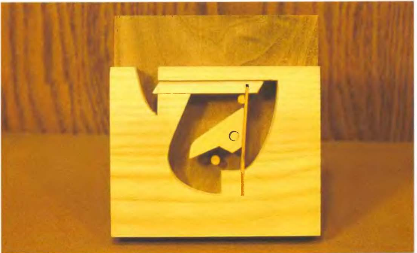
Lock back and center lamination with all interior parts.
