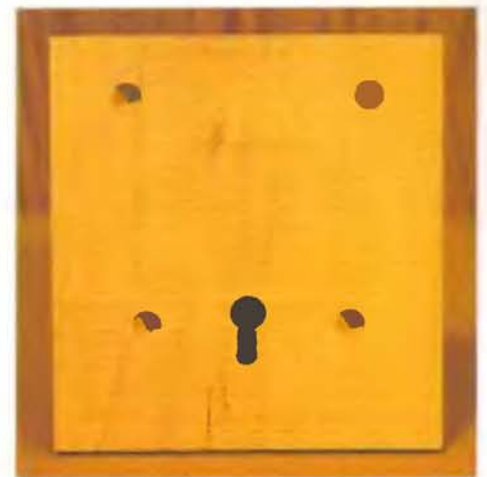
Face lamination with all holes bored out.
