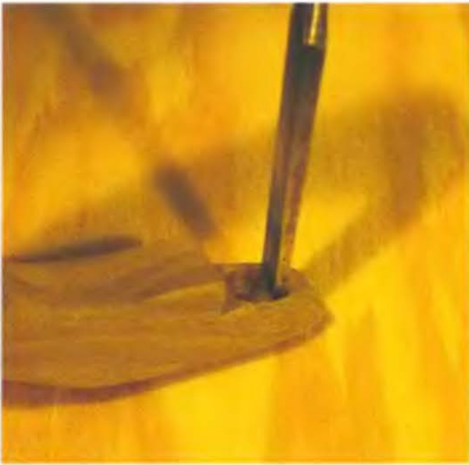
Using chisel to enlarge locking notch.
