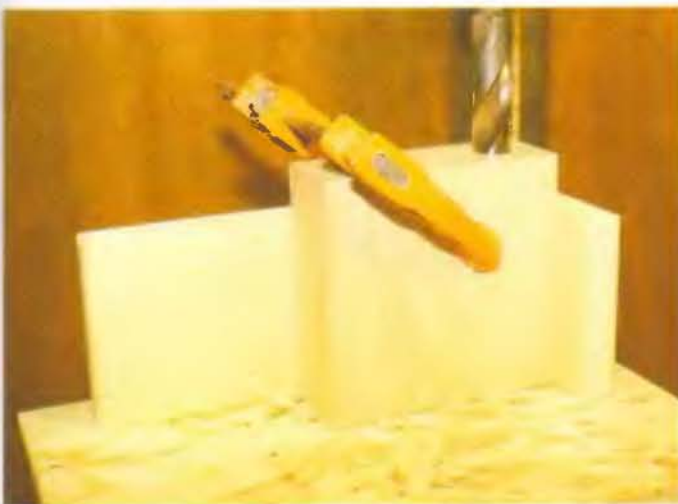
Lock body clamped to drilling platform, drilling shackle hole.
