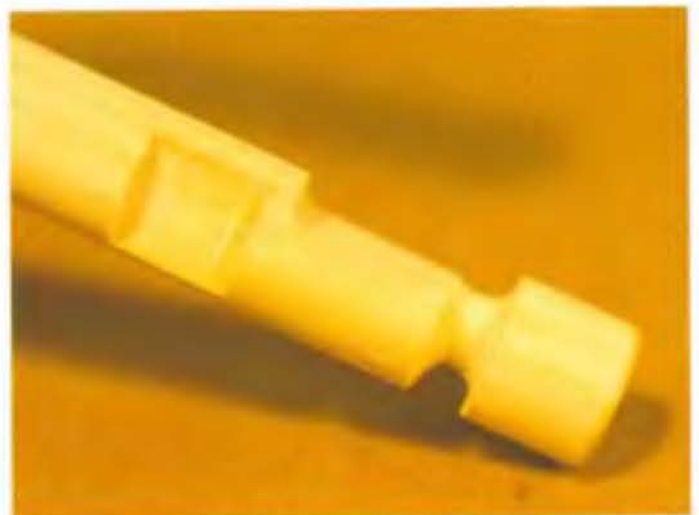
Shackle notched and ready to finish.
