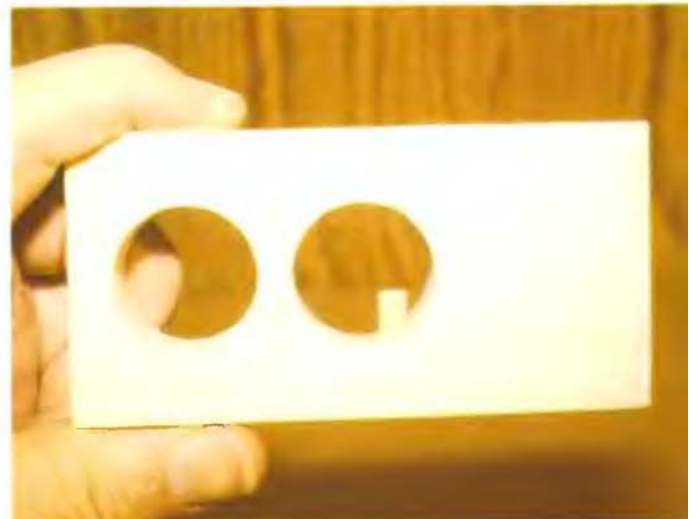
Lamination #3 showing key stop dowel.
