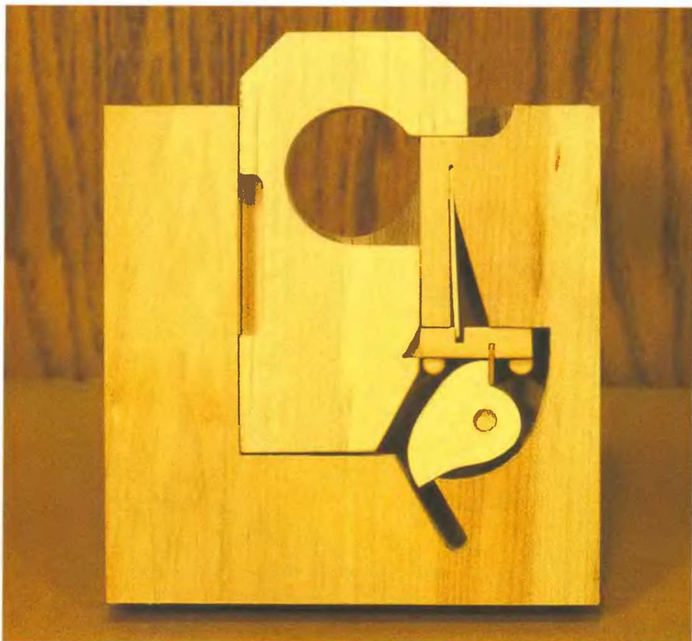
Lock back and center laminations with all interior parts.
