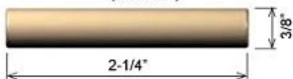
7. AXLE \frac{3}{8} " DIAMETER X 2\frac{1}{4} " (Make 2)
