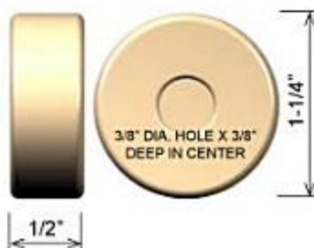
8. WHEEL \frac{1}{2} " X 1\frac{1}{4} " DIAMETER (Make 4)
