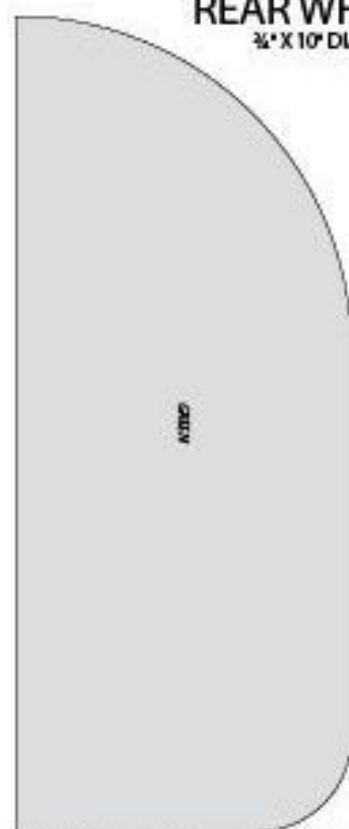
REAR WHEEL SPACER \frac{3}{4} " X 3 \frac{1}{2} " X 8 \frac{1}{2} " (2 REQ'D)
