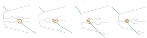
Fig. 1: Closing a crimp bead
